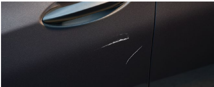
1 dent (greater than 4") or 1 scratch (equal to or greater than 6") per panel
