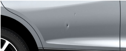
4 or more dings per panel or multiple dings equal to or greater than 2" per panel
